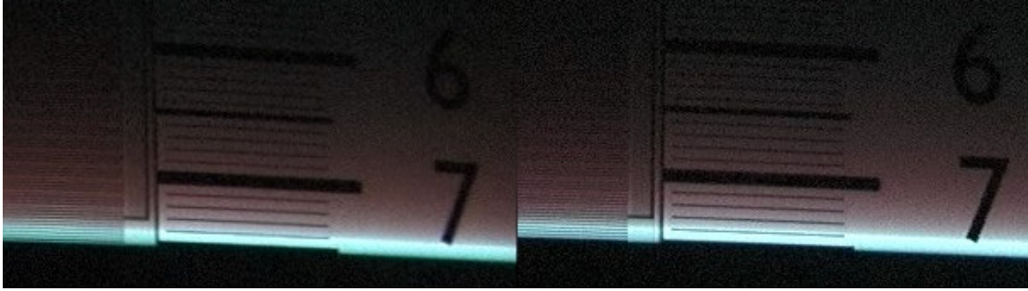
Figure 15. Video frames of two camcorders when the measured time disparity was 2\mu\text{s} .
