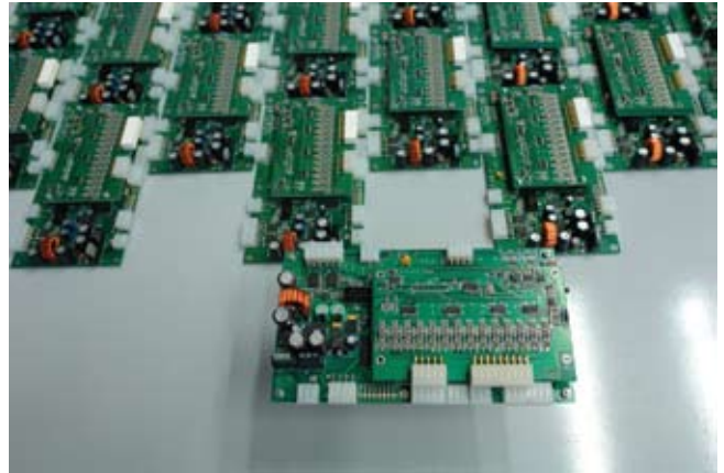
Figure 4: SmartModule - an Air Delivery Control System intended for the control of air flow in the fuel-cell and natural-gas reformer based on a co-generation heating/power supply system
