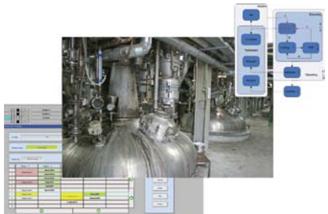
Figure 5: Resin-synthesis batch-process control system based on the PLCbatch tool
