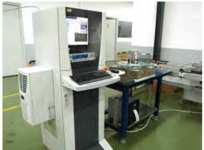
Figure 5: Diagnostic system for electronically commutated motors.
