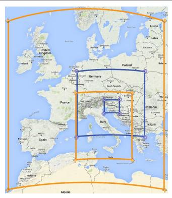
Fig. 2 Larger and smaller geographical domains used in WRF (areas with circles in corners) and QualeAria (areas with crosses in corners) model (Google, 2016).
