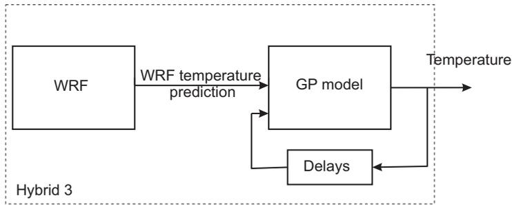
**Fig. 4** Hybrid model of the WRF ARW model and statistical model using temperature-prediction time series and WRF temperature predictions only – Hybrid 3. The statistical part of this hybrid model is trained with temperature measurements and WRF predictions of temperature.
