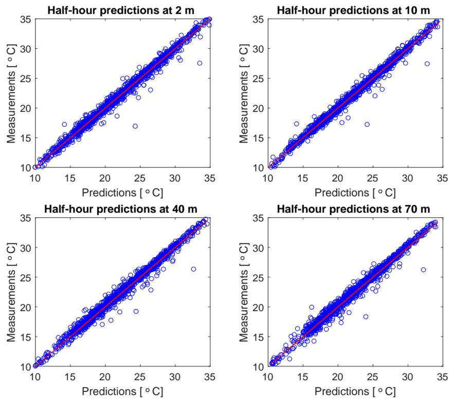
**Fig. 6** Comparison of scatter plots for temperature half-hour-ahead predictions vs. temperature measurements for the period of 30 days at heights 2 m, 10 m, 40 m and 70 m, respectively with the hybrid model of Figure 2. The red line shows the line of ideal match between hybrid-model temperature forecasts and temperature measurements.
