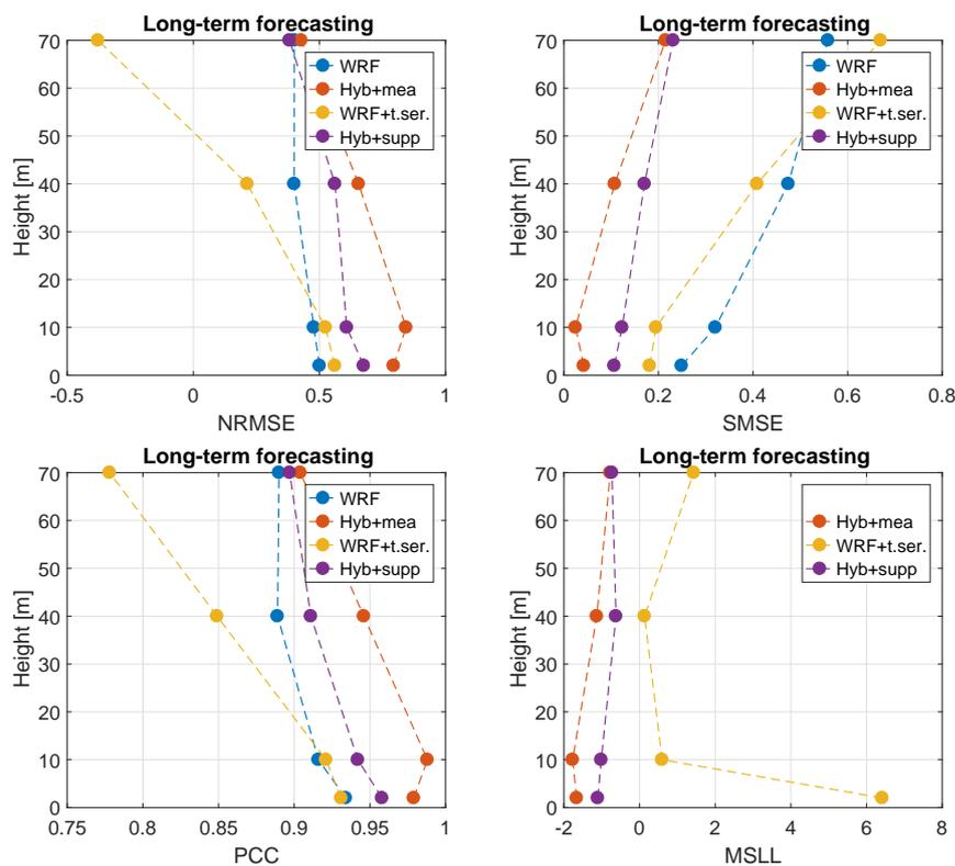
**Fig. 10** Graph for comparison of performance measures for long-term forecast up-to 5 days vs. investigated heights. The performance-measure values are depicted as solid dots, while interpolation lines are depicted with dashed line to illustrate the trend of performance-measure value changes with height.
