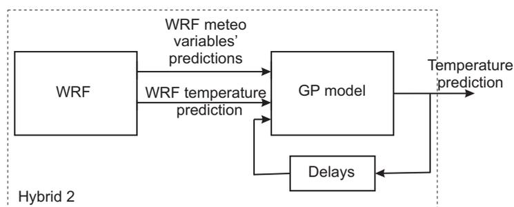
**Fig. 3** Hybrid model of the WRF ARW model and statistical model where the statistical part of the model uses WRF predictions to replace measurements from measurement stations in each time step – Hybrid 2. The statistical part of this hybrid model is trained with temperature measurements and WRF predictions of all relevant meteorological variables.
