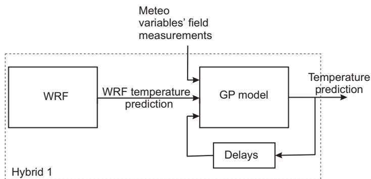
**Fig. 2** Hybrid model of the WRF ARW model and statistical model trained with measurements from available measurement stations – Hybrid 1. This hybrid model requires measurements of meteorological variables for making forecasts in each time step.
