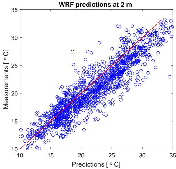
**Fig. 5** WRF temperature forecasts (blue circles) vs. temperature measurements for the period of 30 days at the height of 2 m in the location of Krško NPP. The red line shows the line of the ideal match between forecasts and measurements.
