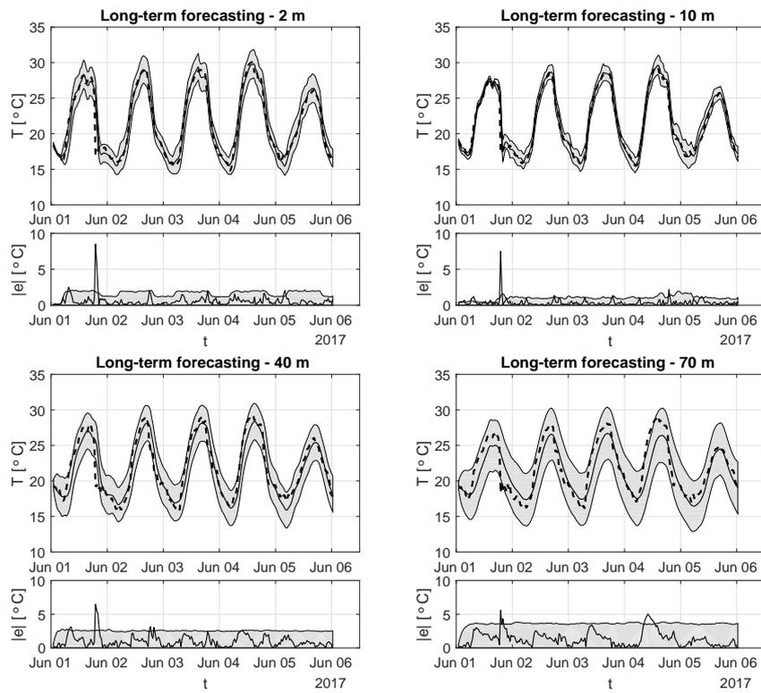
**Fig. 8** Comparison of time responses for long-term forecasts of temperature for the period up-to 5 days at heights 2 m, 10 m, 40 m and 70 m, respectively. Legend: mean values of forecasts – full line in upper figure, 95 % confidence interval – grey band in upper figure, measurements – dashed line in upper figure, the absolute value of the difference between forecasts and measurement – full line in the bottom figure, 95 % confidence interval – grey band in the bottom figure.
