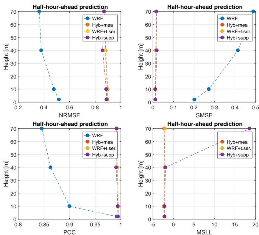
**Fig. 9** Graph for comparison of performance-measure values for half-hour-ahead predictions vs. investigated heights. The performance-measure values are depicted as solid dots, while interpolation lines are depicted with dashed line to illustrate the trend of performance-measure value changes with height.
