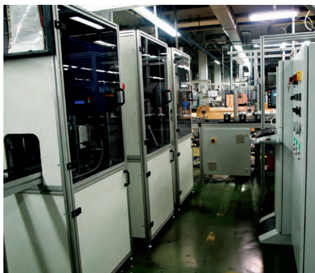
Figure 6: Diagnostic system for end-quality control on the production line for electrical motors of type 462 at Domel d.o.o.
