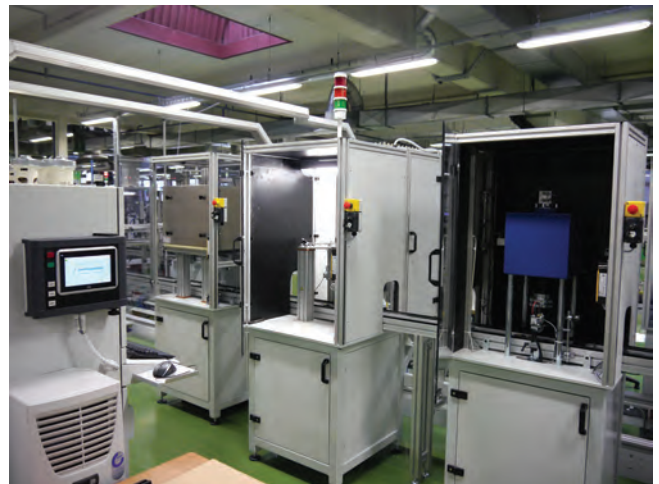
Figure 4: Diagnostic system for the total quality control of eco-motors on the new production line ML-13 in Domel d.o.o.
