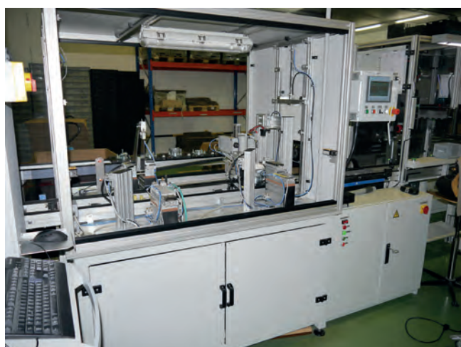
Figure 3: Diagnostic system on ML-14 assembly line at Domel d.o.o.
