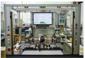
Figure 4: Diagnostic system for End-of-line control of electric drives for bicycles of the Pedelec type (Pedal Electric Cycle)
