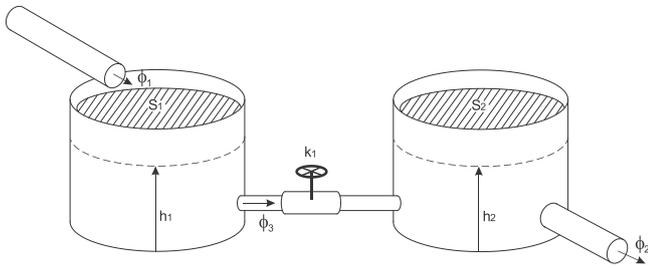
**Fig. 1.** The concept of interacting reservoirs for simplified modelling of relatively flat sewers where backwater phenomena may occur.
